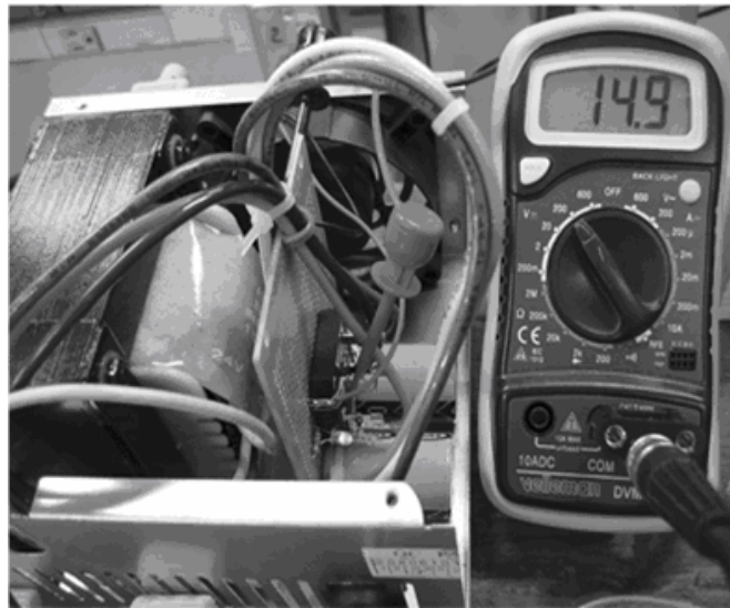
Figure 6.4 The High-Current Power Supply is encased in a metal box with a fan. A multimeter reads the positive DC output of the supply.
